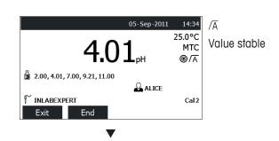
Press **END** to end calibration or repeat the last steps for a multi-point calibration.
