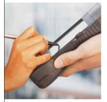
A plug-in prompts the scale operator to have a driver sign an electronic signature pad when a transaction is completed and then adds the signature to the transaction record.
