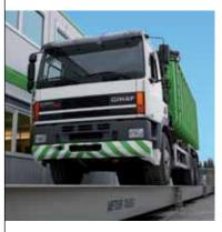
Full-length scales are the first choice for legal-for-trade weighing. Using modular designs, we supply weighbridges to handle even the longest trucks and most complex loading operations. You get reliable weighing, even when dealing with heavy traffic and punishing environments.
