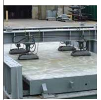
METTLER TOLEDO is the only manufacturer that performs life-cycle testing on actual scale modules. The Module Masher test stand simulates 20 years of truck traffic at full design load. This testing procedure verifies your truck scale's ability to stand up to the real-world demands of vehicle weighing.
