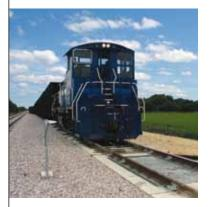
A coupled in-motion (CIM) rail-road track scale is used to weigh rail cars that are coupled together and moving across the scale at speeds of 3 to 5 mph (5 to 8 km/hr). It makes weighing quicker and safer by eliminating the need to uncouple each rail car and position it on a static scale.
