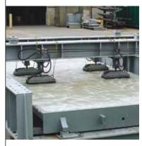
METTLER TOLEDO is the only manufacturer that performs life-cycle testing on actual scale modules. The Module Masher test stand simulates 20 years of truck traffic at full design load. This testing procedure verifies your truck scale's ability to stand up to the real-world demands of vehicle weighing.
