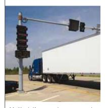
Multi-platform scales use a series of independent platforms to determine individual axle weights and gross vehicle weight. They provide both legal-for-trade weighing and a quick, one-step method of verifying that trucks comply with highway weight limits.
