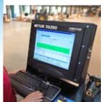
with a user-friendly work-station. Data collection is initiated by scanning the bar code. The data is instantly displayed on the monitor and a traffic light shows the status of the measuring process. The operator has full control at all times, of both current and historical data on the screen.
