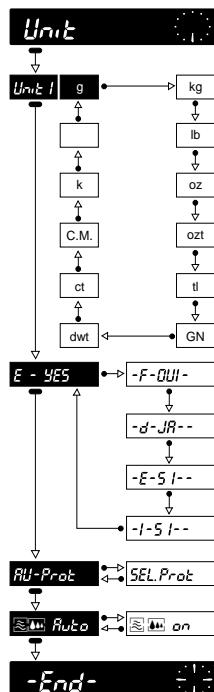
The configuration register with NetEasy-M is distinguished from the configuration register of the balance or scale with the standard program cassette only in the –Unit– sector. With NetEasy-M the following can be selected in the –Unit– sector.
