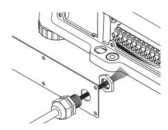
To connect the cable of the power supply unit and the grounding cable proceed as follows:
