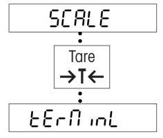
Now press the "Tare" ("No") key repeatedly until the block appears in which you wish to make a setting (in this example the main block "Terminal").
