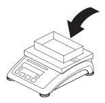
Place the **empty** weighing container or the packaging material on the platter.
