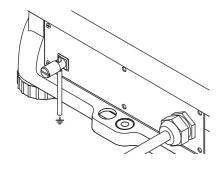
Replace the back plate and fasten it with the screws. When doing so, take care not to trap any wires.
