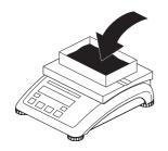
Place the weighing sample on the platter ...
