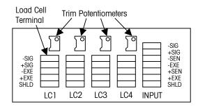
Figure 3-1: Junction Box PCB Layout
