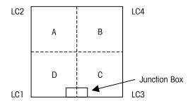
Figure 4-1: Top View of Scale
