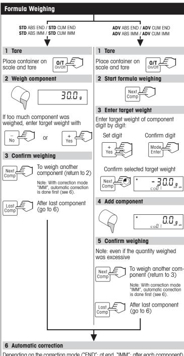
Depending on the correction mode ("END": at end, "IMM": after each component) the scale checks automatically whether extra quantities of components weighed so far must be added.
