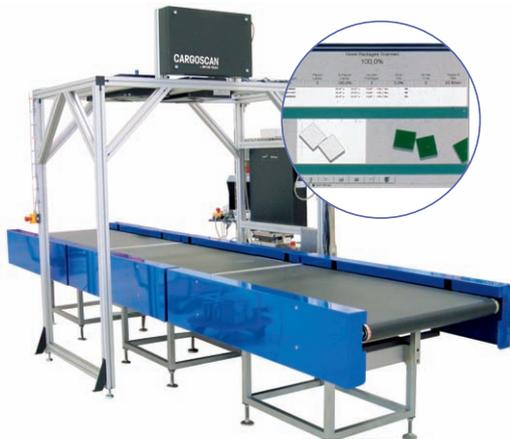
The CS9000 GC is a complete, in-motion data capture solution. Packages, travelling at speeds over 70 m/min are automatically spaced, then accurately, dimensioned, identified and weighed. The information supplied by this system can increase revenues, optimise control of inventory, save on operational costs and improve flow of goods.
