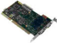
The software on the weighing interface WI-ISA is responsible for the communication between the scale and the PC-based scale driver program. The software itself is located in an Electrically Erasable Programmable ROM (EEPROM). This technology makes it possible to download a new release direct from the ID20 harddisk into the weighing interface without opening the terminal.
