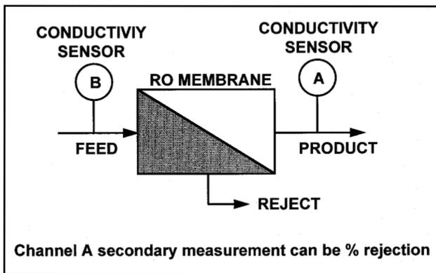
rejection measurement, the product monitoring sensor must be installed in the channel that will measure percent rejection. If the product conductivity sensor is installed in channel A, then percent rejection must be measured
