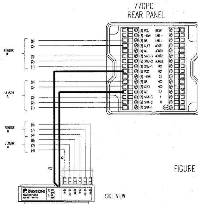
FIGURE 1. 24VDC-Powered Sensor Connections
