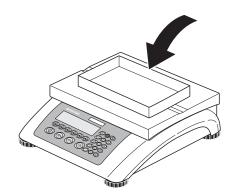
Place the **empty** weighing container or packaging on the scale and then press the  $\leftarrow$  Y  $\leftarrow$  » key briefly, or press the  $\leftarrow$  PT» soffkey if a **known tare weight** has already been established.
