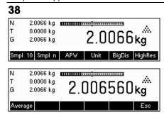
Press the **«HighRes»** softkey in order to display the net weight at a higher resolution.
