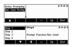
"Def. User Prompt" function allows the user to define a step-by-step flow process. Afterwards, choose "Step 1". A text can now be entered for the user (working instructions) and the corresponding function can be defined.
