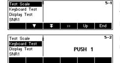
In order to check if all the keys are functioning properly, press **Yes** to start the keyboard test.
