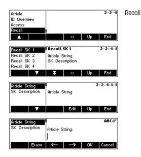
This function allows recalling of an article directly from the database via a softkey. This means a previously defined article can be loaded by pushing one key
