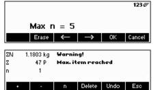
Press the  $\mbox{\ensuremath{\mbox{\bf n}}}\mbox{\ensuremath{\mbox{\bf v}}}$  softkey to limit the number of lots to accumulate.
