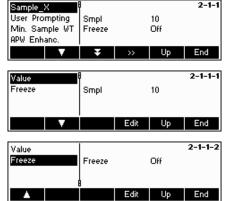
Press « >>> to change the settings into the desired number of pieces or to freeze the actual setting of the Smpl X value.
