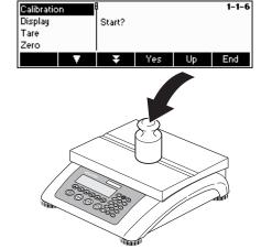
After choosing the calibration weight, place the weight on the weighing pan
