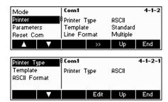
The current printer settings are displayed on the right side of the screen. Press « by to go to the printer settings menu.
