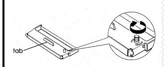
Insert the cartridge as shown below, making sure it snaps in place. The ribbon must be between the printhead and platen. Turn the knob to take up any slack. Close the printer cover.
