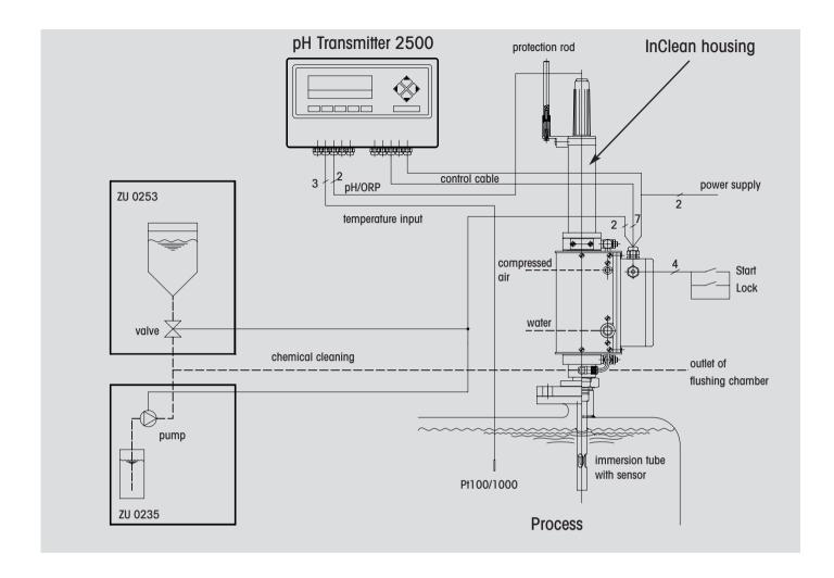
InClean is a measuring system for the pH and Redox measurement with an automatic sensor cleaning function. With this system, increased lifetime of the sensor and decreased maintenance effort can be achieved. InClean adapts to every measuring site where sensor contamination is a problem. The following cleaning cycle can be started automatically or by remote control:
