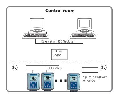
Electrical connection between module and Foundation Fieldbus is in accordance with FISCO (Fieldbus Intrinsically Save Concept, www.fieldbus.org).
