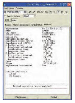
Each AI TB of the FF module has a ring buffer which can store up to three protocols. A fourth protocol would overwrite the first protocol in that TB.
