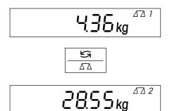
The scale symbol in the upper right corner of the display indicates the currently active scale ( $\Delta \Delta 1$  or  $\Delta \Delta 2$ ).
