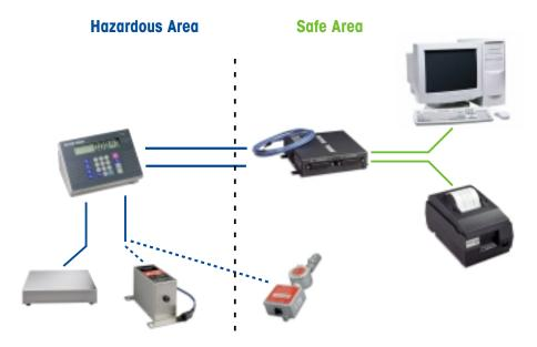
sically safe AC power supply is suitable for Class I, II or III, Division 1 or 2, Groups C, D, E, F or G areas. When located in a safe area, the AC power supply can power the intrinsically safe terminal in a Class I, II or III, Division 1 or 2, Groups A, B, C, D, E, F or G area.
