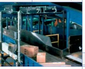
The CS5200 Measuring Beam provides a fast, simple and accurate method for measuring your objects without invading existing conveyer systems. The CS5200 Measuring Beam is a Over-the-Belt-Dimensioner that use Cargoscan's patented and well proven PILAR ® technology, offering you benefits such as:
