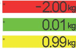
Over/Under Checkweighing ICS466x
