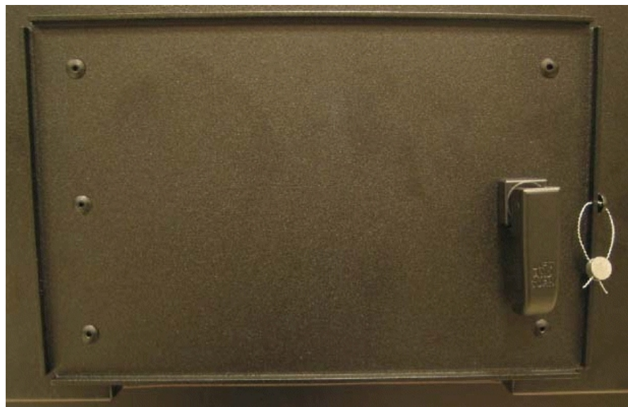
Typical sealing / Scellage typique
