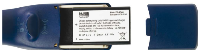
Figure 5: Installing the main battery
