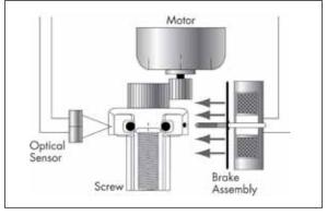
Figure 4- Mechanisms of a DC motor system
