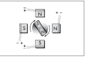
Figure 2- Multiple stators
