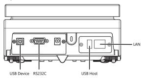
Interfaces and possible connectivity of peripheral devices:
