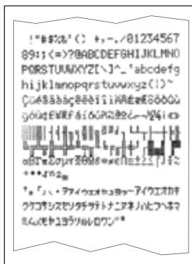
The BT-P42 is equipped with a self-test which automatically prints out the character set of the printer.
