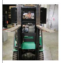
The center of the carriage is open, providing a high-visibility window. This design makes it easy for the forklift operator to see loads, position forks for lifting and avoid accidents.
