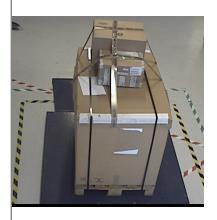
Take a picture of each pallet for proof of condition, content and measurement using a legal for trade system.
