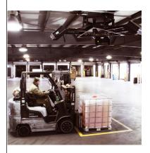
Simply place the pallet underneath the dimensioner and trigger measurement using your preferred method of identification.
