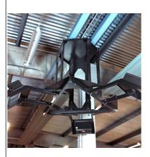
Out of the way of forklift traffic, the overhead mounting makes it easy to position pallets under the dimensioner with no slow-down in operation.
