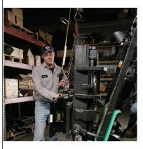
The VFS220 scale carriage can be installed in 30 minutes. It is ready for weighing immediately. Just hang the scale on the lift bracket, adjust the locating tab and tighten.
