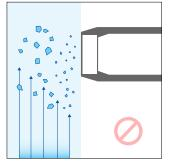
Figure 2: Non-ideal orientation— Probe window flush with the pipeline or reactor wall
