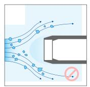
Figure 4: Non-ideal orientation— Probe window as flat obstruction to the flow of material
