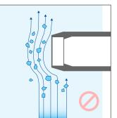
Figure 3: Non-ideal orientation— Probe window parallel to the flow of material
