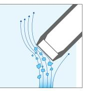
Figure 1: Ideal probe orientation— Probe window at a 30° to 60° angle to the flow of material
