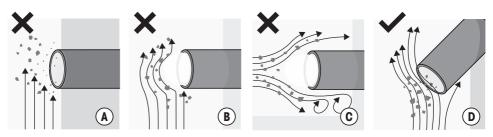
**Figure 5.** Implementation of a ParticleTrack instrument: (A) flush with wall of vessel or pipeline; (B) inserted tangentially to process flow; (C) inserted perpendicular to process flow at an elbow; and (D) inserted at optimal angle (45°) relative to process flow.
