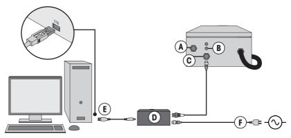
Figure 6. Instrument connections: (A) Power; (B) Air inlet for probe scanner; (C) Fiber communication connection; (D) Fiber-to-USB extender; (E) USB cable; (F) Extender power supply
