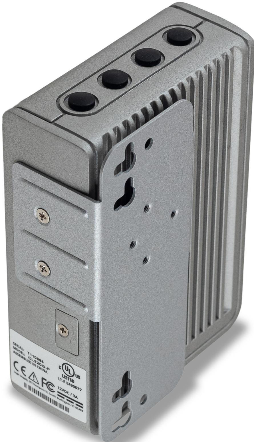
Figure 65: Mounting Bracket Attached to ACI400
