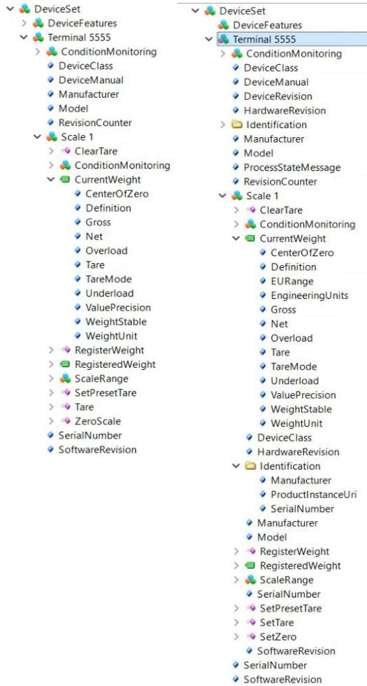
Figure 53: Original (left) and Standard (right) OPC UA Data Structure Tree
