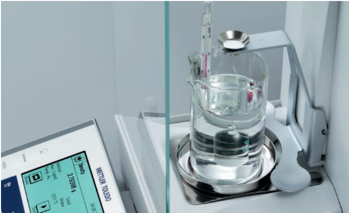
Where required, the thermometer and glass sinker are available in certified versions.
