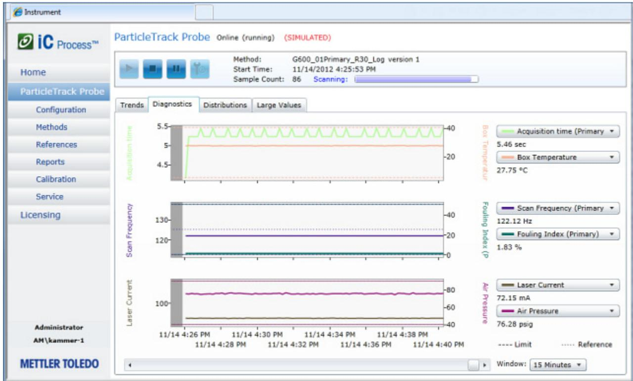
Figure 6-6 Diagnostic tab (with instrument online)
