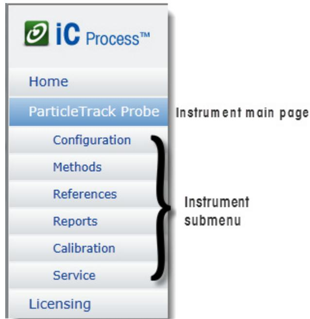
Figure 4-23 Instrument submenu on left navigation menu
