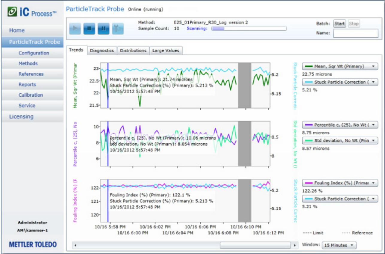
Figure 4-16 Reader bar in stacked trend view
