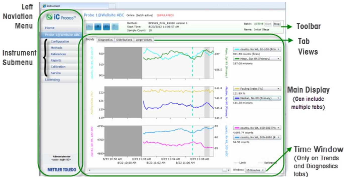
Figure 2-2 iC Process main instrument display—labeled
