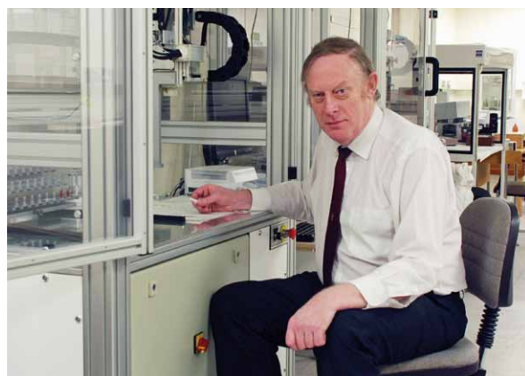
John Pain with the new microgram weights and METTLER TOLEDO’s ‘a5’ comparator
