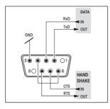
Every balance can be equipped with an optional RS232C interface for connection to a peripheral device (e.g. printer, auxiliary display or PC with a 9-pin male connector, see Section 6.4). The balance must then configured to suit the peripheral device in a menu dialog (Sections 4.3.8 - 4.3.13).
