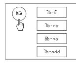
7b-E 7 data bits/even parity 7b-no 7 data bits/no parity 8 data bits/no parity 8b-no 7b-odd 7 data bits/odd parity
