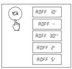
Automatic shutoff after 10 minutes inactivity A OFF 10' A OFF -Automatic shutoff not activated A.OFF 30" Automatic shutoff after 30 seconds inactivity A.OFF 2' Automatic shutoff after 2 minutes inactivity
