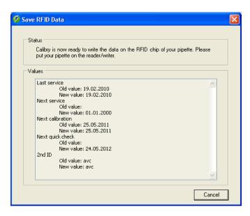
The calibration procedure itself is the same as for conventional pipettes. Once the calibration is complete, Calibry will indicate that the data is now ready to be written to the pipette's RFID chip. The data to be transfered will be displayed at the bottom of the dialog.
