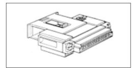
Page 2: As mentioned in the Description overleaf, scales to types PJ12, PJ15 and PJ1220 DeltaRange® are already factory-fitted with the bidirectional data interface. There is therefore no need to fit an extra PCB, one simply has to to insert the 019 Option (special program cassette). This is done in the following manner:
