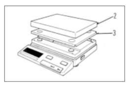
Lift off load plate 2 and load support 3.
