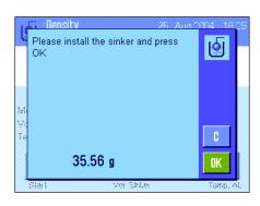
Press the "**Start**" function key to start the density determination. You are then prompted to install the sinker (weighing in air for taring).
