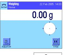
On Off Switching on the balance: Press the «On/Off» key briefly. The balance carries out a test and is then ready to weigh.
