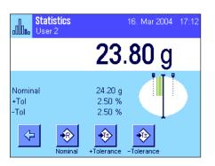
As soon as the nominal value and tolerances have been entered, a graphic weighing-in aid ("SmartTrac") appears in the display with tolerance markers, which simplify weighing in to the nominal value. You can roughly weigh in your samples until the lower tolerance value is reached and then accurately dose, if necessary, up to the nominal value.
