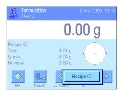
If you are working with a weighing container, place it on the balance and press the « $\rightarrow$ T $\leftarrow$ » key to tare the balance.
