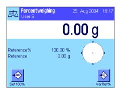
After you have selected the application, the display shown at left appears. Some of the special function keys and the special information fields for percent weighing are activated at the factory. How you can adapt these and other settings to your needs is described in the Sections that follow.
