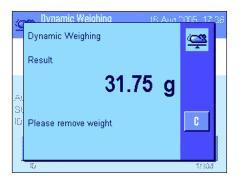
When the weighing is finished, the result is displayed along with a prompt to remove the weighing object.
