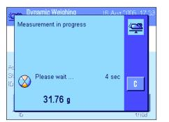
Place the weighing object on the balance. The weight of the weighing object must be greater than the weight shown in the "AutoStart" information field, otherwise the weighing cycle will not start automatically. After the automatic start, the window shown at left appears.
