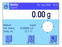
In the application-specific settings for the method, select "Liquid" (Section 13.3.2).
