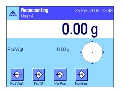
The display opposite appears when the application is selected. Some of the special function keys, as well as a special information field for piece counting, are activated ex works. The function keys and other settings can be adapted to your requirements, according to the descriptions in the following Sections.
