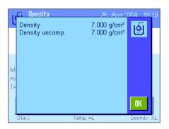
The weighing result is saved and you are then prompted to immerse the solid body in the auxiliary liquid.
