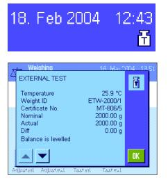
Pressing this function key checks that your balance was adjusted correctly using an external weight. This can be implemented at any time.
