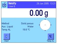
In the application-specific settings, select **"Solid porous**" as your method (Section 13.3.2), and specify the desired auxiliary liquid (Section 13.3.3).
