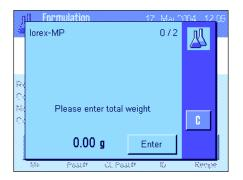
Depending on the basis for weighing in components, which is specified in the formula definition (Section 10.5.2), when the formula is called up you will first be prompted to enter the desired **final weight of the formula** or the **nominal weight of the first component**. Enter the required value.
