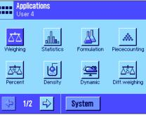
**Selecting the application:** If you do not wish to work with the current application, select the application menu using the «**EXERP** key (alternatively you can touch the relevant zone in the top left of the display). Touch the icon for the desired application and the software loads the selected application.
