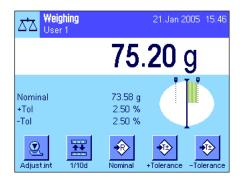
As soon as the nominal value and tolerances have been entered, a graphic weighing-in aid ("SmartTrac") appears in the display with tolerance markers that simplify weighing in to the nominal value: You can roughly weigh in your samples until the lower tolerance value is reached and then accurately dose, if necessary, up to the nominal value.
