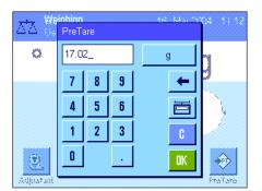
To enter a tare preset, the relevant function key must be activated (Section 8.2.2). When the function key is pressed, the window for entering the tare value appears.
