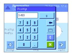
If the piece weight is known, it can be entered directly. To do this, press the "PcsWgt" function key. An input field appears, in which the piece weight can be entered in the desired unit.
