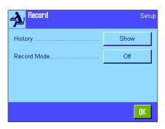
The balance can document modifications to protected settings. A list of these operations can be viewed in the "Record" menu and recording can be switched on or off.
