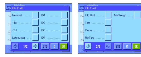
This menu can be used to specify which information fields are to be displayed. The fields assigned a number will be displayed in the application. The numbers determine the order of the information fields in the display. **Important:** For reasons of space, a maximum of 4 information fields can be activated. When an information field is activated or deactivated by touching it, the order of the fields is updated automatically.
