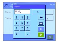
To enter the weight value, press the corresponding button. A numeric input field appears, in which the tare value can be entered. **Note:** Instead of typing in the value, you can place the relevant tare container on the weighing pan and then press the button with the balance icon. The measured weight value is thus transferred directly. Notes on working with the tare memories can be found in Section 8.3.2.
