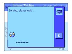
When you remove the weighing object (and provided the "AutoTare" function is activated) the display is automatically reset to zero. The balance is then ready for the next weighing.
