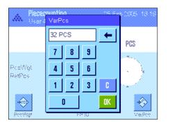
If you have placed a **different number of reference pieces** on the weighing pan than the number corresponding to the "FixPcs" key (e.g., 32 pieces), press the "**VarPcs**" (variable piece number) function key. An input field appears, in which you can enter the number of pieces.
