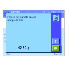
If you are using water or ethanol as the auxiliary liquid , enter its temperature using the "Temp. AL" function key. Density tables for these two substances covering the temperature range from 10 °C to 30 °C are stored in the balance; see also Sections 13.7 and 13.8). The illustration here shows the corresponding input field (input in °C with 1 decimal figure).
