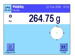
**Zeroing:** A new zero point is set using the  $\ll \rightarrow 0 \leftarrow \gg$  key and all weight values (including the tare weight) are measured in relation to this zero point. After zeroing, the following values apply: tare weight = 0, net weight (= gross weight) = 0. Always use the  $\ll \rightarrow 0 \leftarrow \gg$  zeroing keys before you start with a weighing, especially before recording a tare weight (using the  $\ll \rightarrow 1 \leftarrow \gg$  key).
