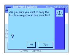
When the function key is pressed, the prompt opposite appears. When you respond with yes, the tare weight of the first sample is copied for all further samples in the current series (as long as no tare weight has already been defined for these samples).
