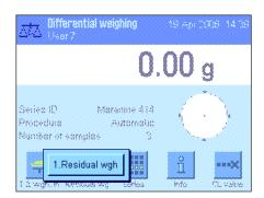
When the balance has determined the tare weight, you are prompted to begin weighing. To perform weighing in, add the weighing sample to the container and then press "**OK**". While the balance is determining the weight, a corresponding message is displayed.
