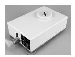
You can also clean the load cell using a **low-pressure hand sprayer**. Before using a sprayer, remove the weighing pan and seal off the weighing pan retainer with the white plastic cover (A). Make sure that the cover locks on properly! The connector cable to the electronic unit must be securely screwed on to ensure that the jack (B) is sealed. Under these conditions, the load cell meets IP45 requirements. After you have cleaned the load cell, dry it off with a soft cloth.
