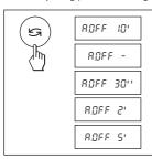
A.OFF 10' Automatic shutoff after 10 minutes inactivity
