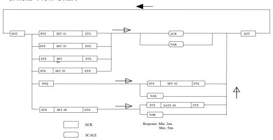
Note: The scale replies to ENQ with NAK when there is no load on the platter, the scale is in motion, under zero, or overcapacity. NAK is sent in response to the setting strings if there is invalid data in the setting.
