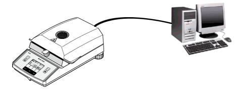
The standard configuration of MJ33 is: 2400 baud, 7 bits, even parity, no handshake. These settings may be adjusted in the menu of MJ33. Additionally the printout setting in the menu should be "off". This avoids that printout strings are sent to the computer. Please refer to the Operating instruction.
