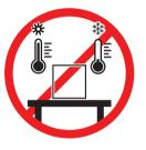
Sufficient spacing for balances: > 15 cm all around the instrument Take into account the environmental conditions. See "Technical Data".
