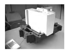
Place the set with the AC adapter in front of the set with the draftshield glasses.
