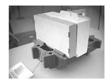
Insert the terminal into the packing cushion as shown in the illustration.
