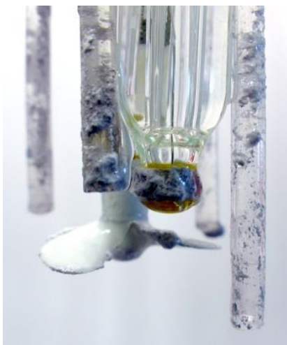
Figure 14. The condition of the sensor after measurement of 15 samples with the "modified" method.
