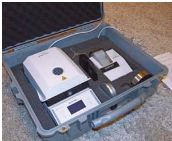
A protective box is designed to protect the HB43-S during travel and placed on the back of NEETRAC's utility trucks.
