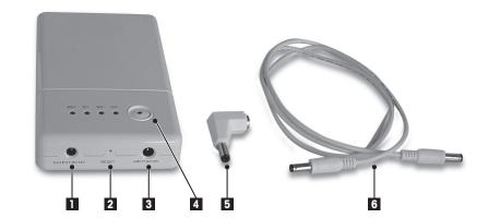
Input / Output To charge the PowerPac, connect the AC adapter of your balance to INPUT (3).
