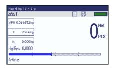
Enter the known tare weight of the container, 0.48 kg for example. Touch keys 0.48 and the TARE key...
