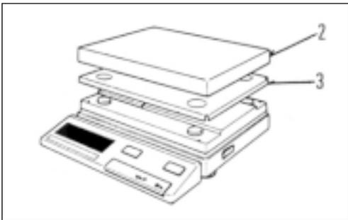
Lift off load plate **2** and load support **3**.
