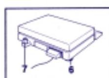
The scale must be relevelled whenever it is moved. To do this, turn the three adjusting feet 6 until the bubble in the level indicator 7 is central.
