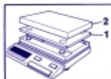
Place plate support 1 and load plate 2 on the scale.
