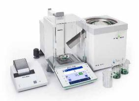
An XPE balance, LV11 automatic tablet feeder and SQC-XPE provide a standalone solution for determining the weight uniformity of tablets, capsules, powders and suppositories in accordance with the European Pharmacopoeia.
