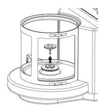
3 Place the weighing chamber plate into the weighing chamber.
