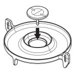
2 Center the drip tray with the weighing pan in the middle of the weighing chamber.
