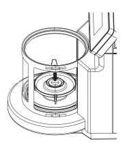
3 Close the weighing chamber and place the draft shield cover glass on top of the weighing chamber.
