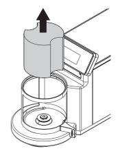
2 Open the weighing chamber door and remove the weighing pan from the weighing chamber.
